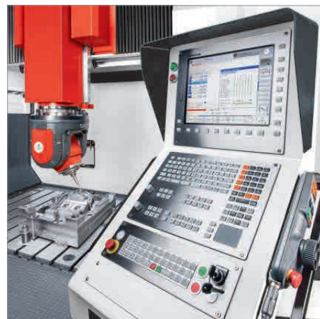
Std. HEIDENHAIN TNC 640 5 axes controller
