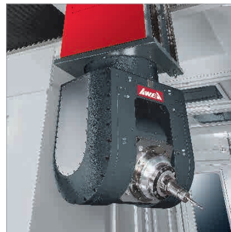
Opt. GERMAN made two axes head (KESSLER)
