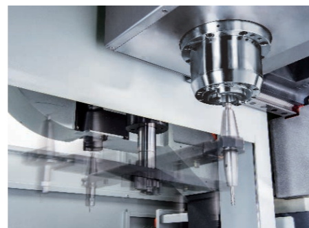
High reliability ATC system
